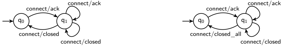
(a) Non-deterministic finite state machine modeling an abstraction of a connection procedure. The model is not observable non-deterministic.
