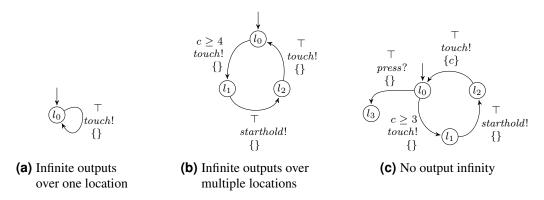
Figure 3.3: Examples of two infinite outputs and one with a clock reset that avoids infinite outputs
