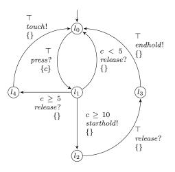
Figure 2.2: This TA is a representation of the Smart Light Switch, which is an adaption of the Touch Sensitive Switch presented by Hessel et al. [24].
