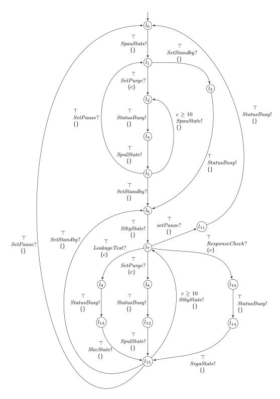
Figure 5.19: TA that models parts of the Particle Counter
