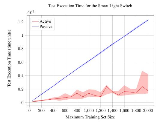
Figure 5.4: Execution time of training set, which is used to learn the TA of the Smart Light Switch using hints
