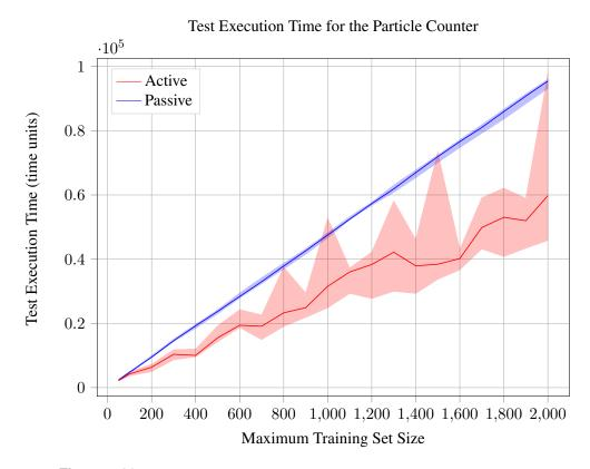
Figure 5.22: Execution time of training set for the Particle Counter using hints
