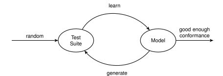
**Figure 3.1:** In recurring order, we learn a model and extend our test suite by newly generated counterexamples. We start with a random test suite and stop learning if we find a model with a good enough conformance.
