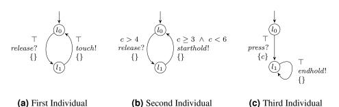
Figure 2.5: Examples of initial population that are created via GP for the learning of the Smart Light Switch of Example 1.
