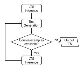
Figure 2.1: General procedure that is used in the iterative refinement approach for LTS proposed by Walkinshaw et al. [53]
