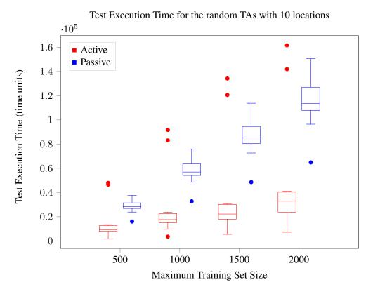
**Figure 5.27:** Execution time of training set, which is used to learn the TA of the random TAs with 10 locations using hints
