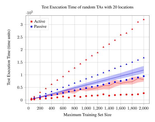
Figure 5.41: Execution time of training sets, which are used to learn the TA of the random TAs with 20 locations using hints
