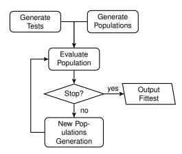
Figure 2.4: Tappler et al. [47] proposes a GP procedure that learns based on a given set of tests. The proposed GP procedure uses two different populations.
