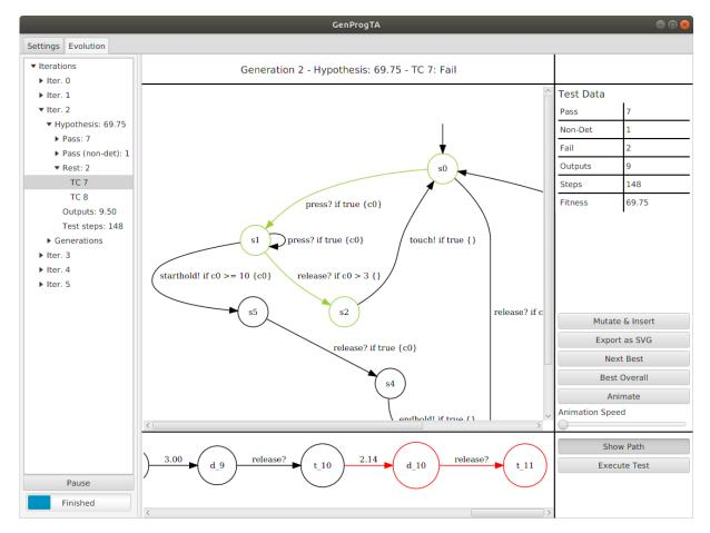
**Figure 4.3:** This evolution view shows the individual iterations of the evolution process. In this view we can monitor every inferred hypothesis and the found counterexamples. It is also possible to execute the counterexamples on the TAs.
